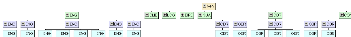
Fig.6 – Acquisition work packages in the schedule now include activities by functional departments, increasing the control over delays in logistics, engineering, quality control, board of directors and other areas that influence the final delivery date of necessary equipment and materials.
